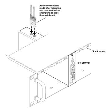
Note: When the REMOTE module is rack mounted, the audio connections must be made after the module has been fixed in place. Access is required to the rear and above the rack. Remember to remove the audio connections before attempting to slide out the REMOTE module.
